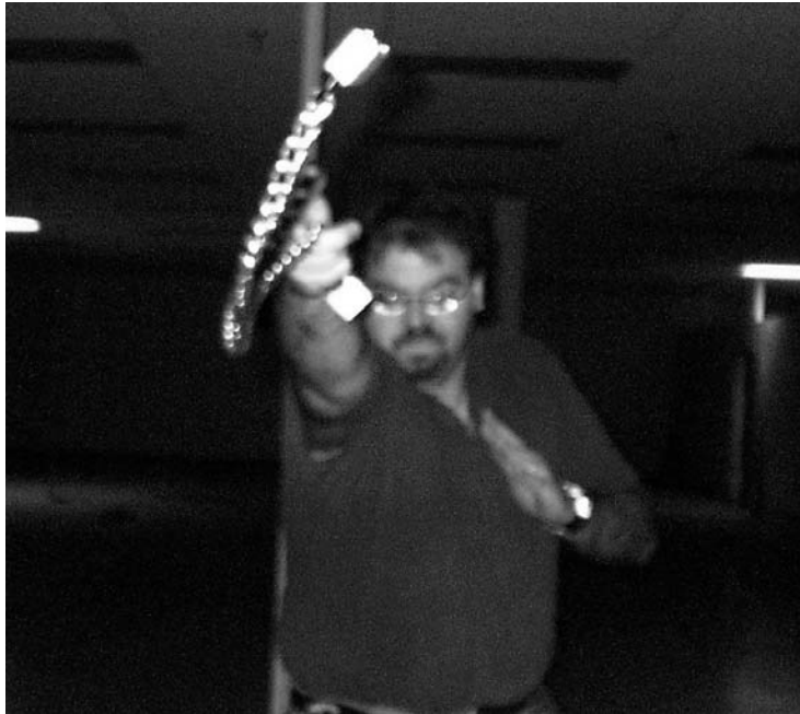
Chain cast immediately after full extension, showing the beginning of the snapback.
